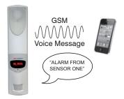
If enabled, Guardpost reports alarms by audible message to up to two telephones via the GSM network.
