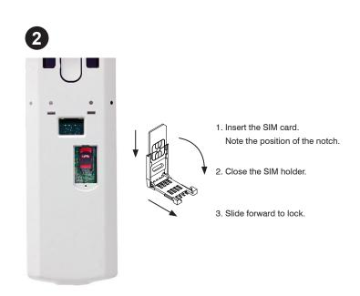
Insert the SIM card as shown then secure the access panel.
