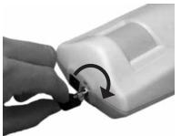
2. To start the unit, turn the main keyswitch clockwise to the ON position.
