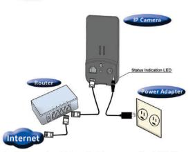
Make sure you correctly plug in the power adapter and the ethernet cable. The IP Camera will get an IP address from your Router automatically. (DHCP must be enabled on the router). The diagram left shows you how to connect the device correctly.
